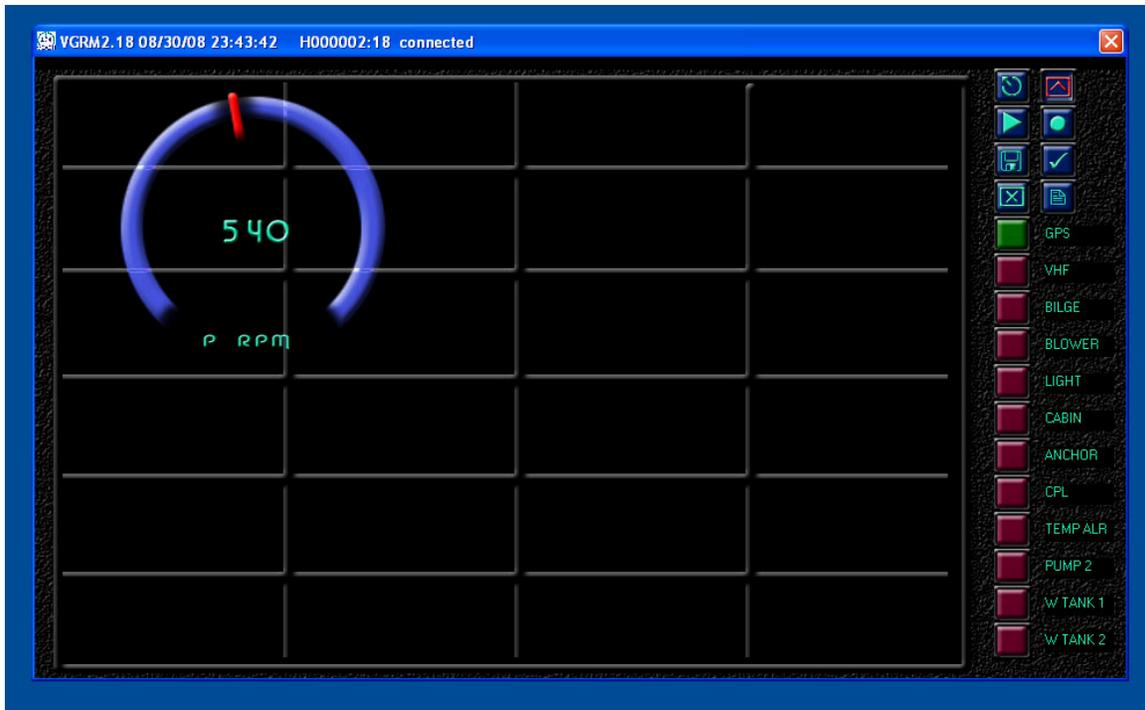
In this example a Digital Dial was chosen to display RPM in the upper right position.
