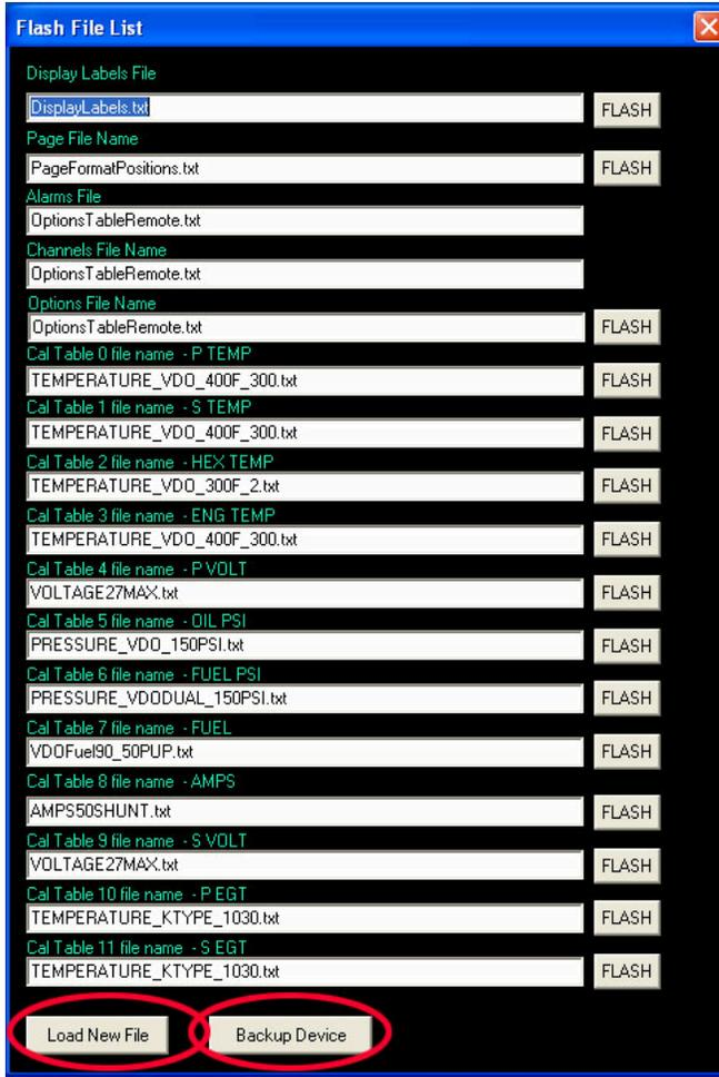
Two buttons **LOAD NEW FILE** and **BACKUP DEVICE** can only be used with a FLASH programming cable to reprogram an attached vGauge or SeaGauge unit.
