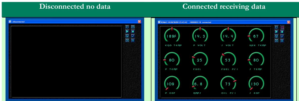
After successful connection the TITLE BAR will display “Connected”. When NMEA data starts arriving the TITLE BAR will display the name of the device sending data vDash will decode compatible NMEA data and display the device labels on the left and sensor data on the right. vDash will display the first 8 characters of device labels and the first 6 characters of sensor data.
